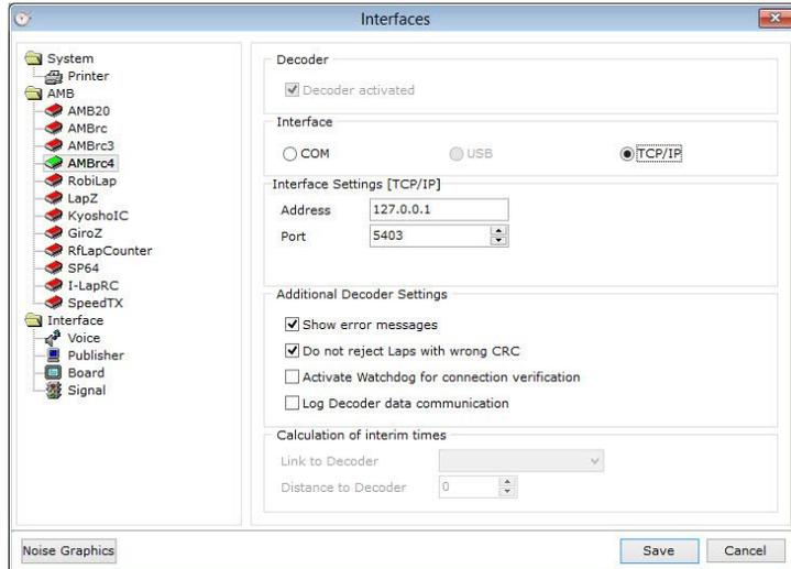
The proper work of the decoder can be checked with the transponder logfile, which can be activated by pressing the F4 key.
