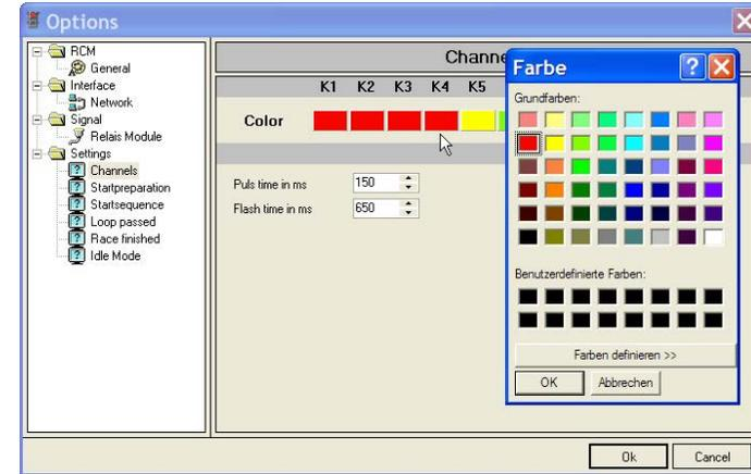
Just click on one of the color fields below the channel numbers K1 to K8 and a color table is opened from which you select the desired color. Below in the window the pulse time for the one time flashing of the lights and the frequency of the continuous flashing (flash time) can be set in milliseconds.
