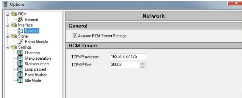
Please leave the number of the TCP/IP Port at 30002. Only with this port RCM Signal is able to receive the necessary information from RCM Ultimate. Confirm your settings by clicking Ok. Now the footer line changes to “Connected to RCM-Signal Interface” and the color of the bar will change to white. Please consider, that it can take several seconds until RCM Signal has found the connection to RCM Ultimate. In the footer line of RCM Ultimate you will find the information “Signal: 1”.
