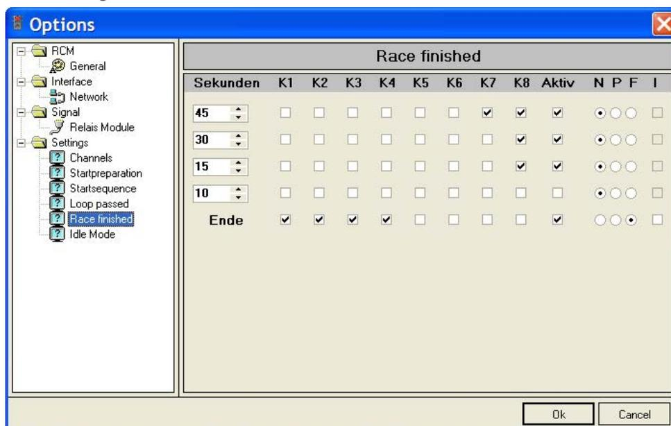
The function for 5 different conditions can be set. In the left column the time before end is set, at which the function is executed. Below the channels K1 to K8 the lights will be activated, which will be switched on or of.
