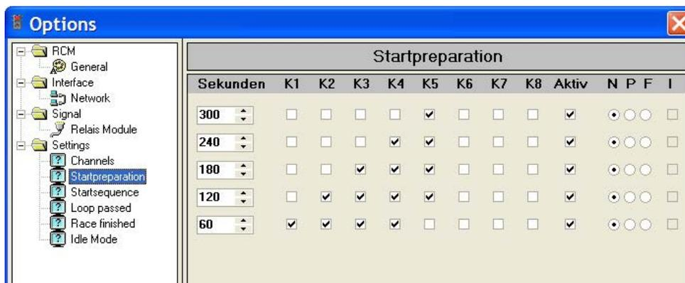
The function for 5 different conditions can be set. In the left column the time before start is set, at which the function is executed. Below the channels K1 to K8 the lights will be activated., which will be switched on or of.
