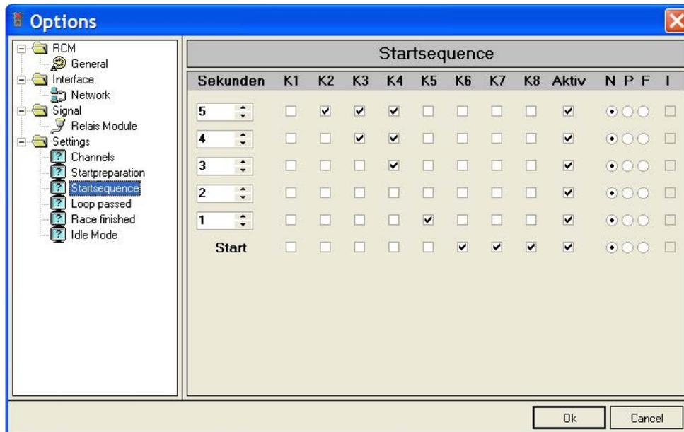
The function for 5 different conditions can be set. In the left column the time before start is set, at which the function is executed. Below the channels K1 to K8 the lights will be activated, which will be switched on or of.
